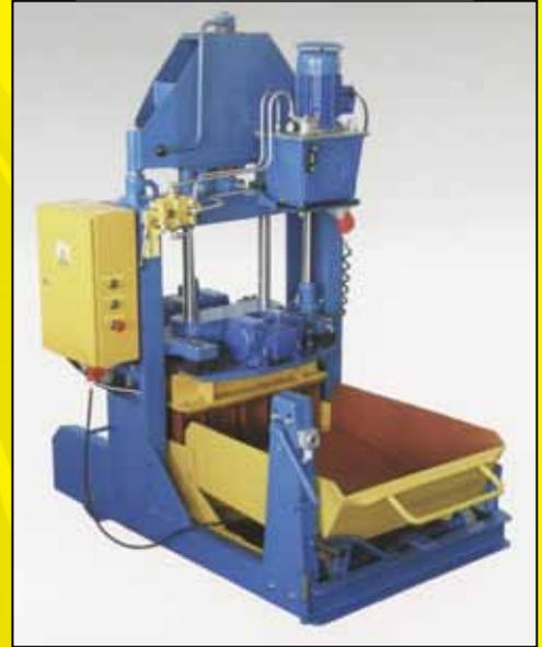
The HK-6 BIS is a small semi automatic block making plant, capacity 1,500 blocks per 8 hour day.
